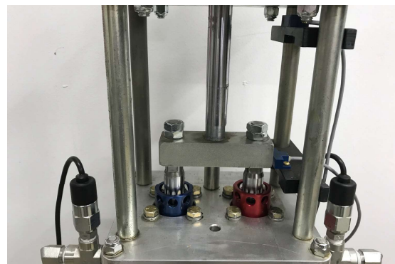
Pumps Shown In Parked Position
