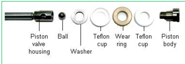
Breakdown of internal foot valve.
