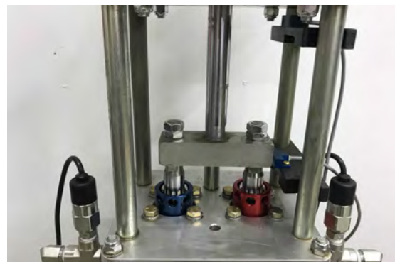
Pumps Shown In Parked Position
