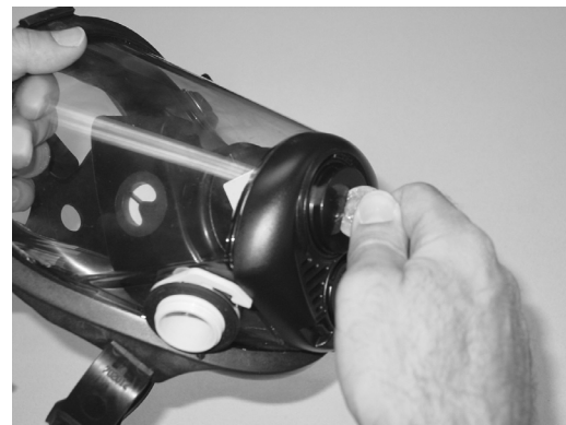
Figure 5. Tighten Nozzle Plug with Coin in Molded Slot
