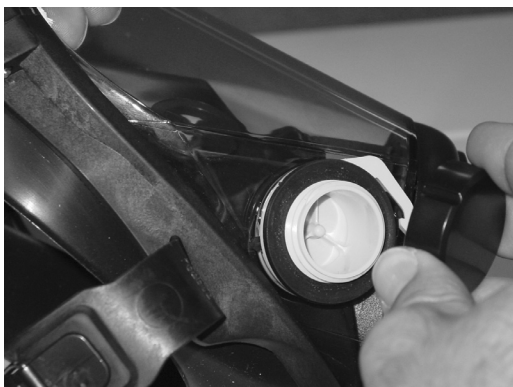
Figure 6. Thread Screw Cap onto Side Connection Port (CF-SAR and PAPR Only)
