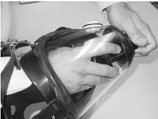
Figure 2. Push Down on Adapter Locking Tab
