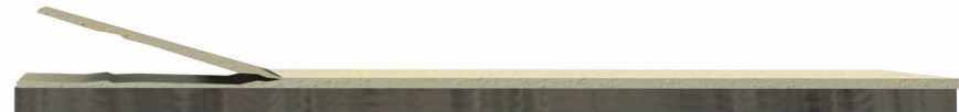
Detail B--Cohesive Failure of Coating: coating breaks within itself and not at the substrate
