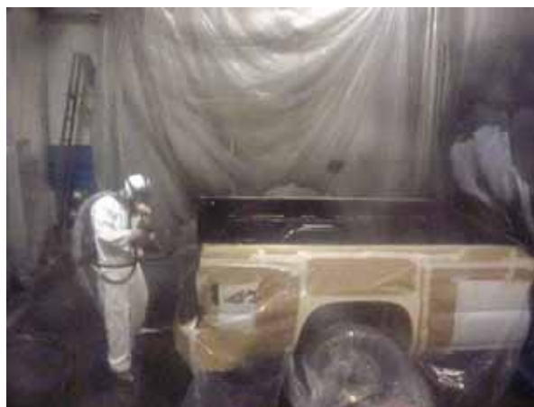
Figure 1. Spraying base coat with protective equipment.
