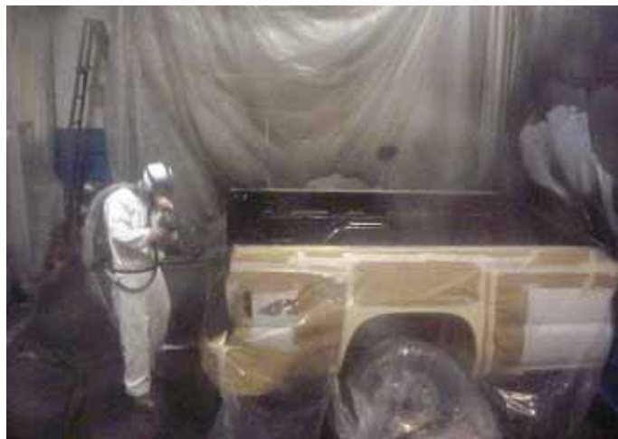
Spraying base coat with protective equipment.
